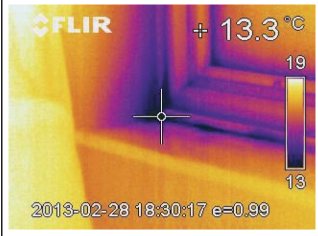
Pictures 14 and 15 showing the significant heat loss paths at the corners of the seemingly well insulated windows.
