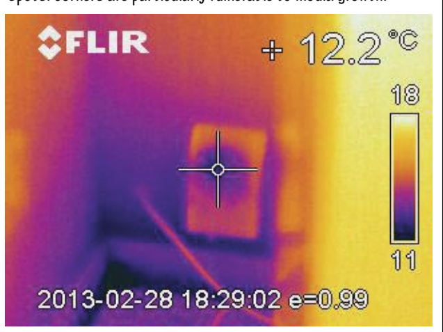
Pictures 7 and 8 show that even socket entry points are cold spots. Corners are particularly vulnerable to mould growth.
