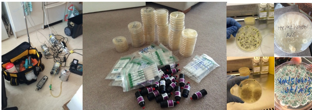
Figure 3: (from left to right) All testing equipment, collected surface and air (both Andersen and NAHA methods) and agar plates at the end of incubation period
